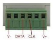
V+ connect strip positive, V- connect strip negative, DATA connect strip data port, CLK connect clock port.
